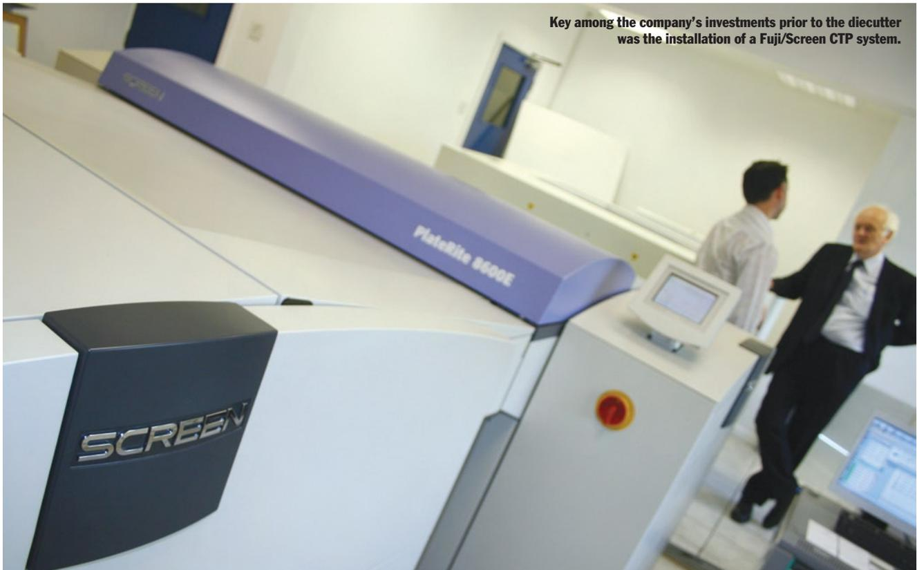
**Key among the company’s investments prior to the diecutter was the installation of a Fuji/Screen CTP system.**
